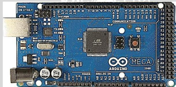
**Gambar 2.6 Arduino Mega 2560**
