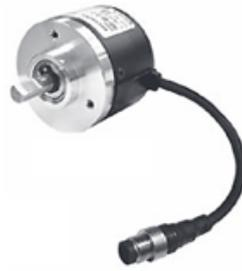
**Gambar 2.5 Increment rotary encoder Autonics E50 Series**
