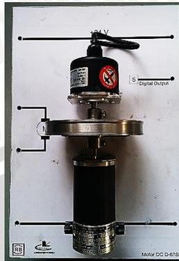
**Gambar 4.7** Modul motor DC D-6759 dan *rotary encoder* Autonics E50S8-360-3-N-24
