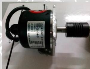
Gambar 4.5 Rotary encoder Autonics E50S8-360-3-N-24
