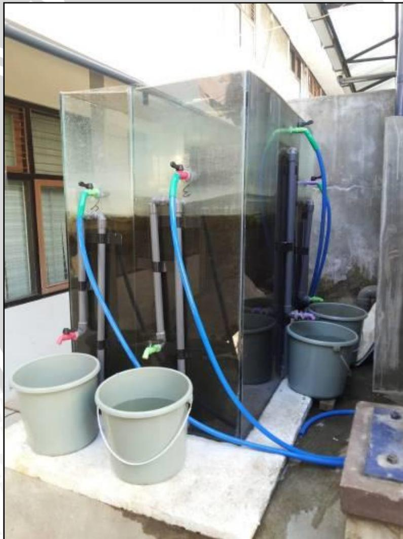
Gambar 3.1. Unit *Biosand Filter*
