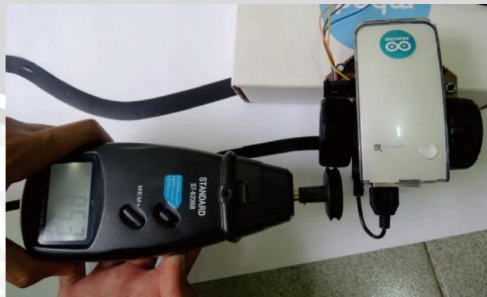
Figure 3.23 Test motor speed using digital tachometer.
