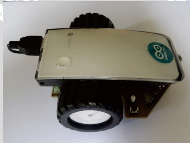
Figure 3.3 Arrow-bot line follower robot overview.
