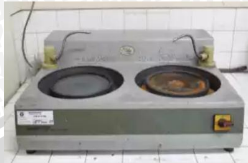
Gambar 3.6 Centrifugal Sand Paper Machine
