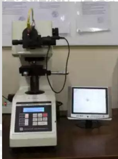
Gambar 3.3 Digital Microvickers Hardness Tester
