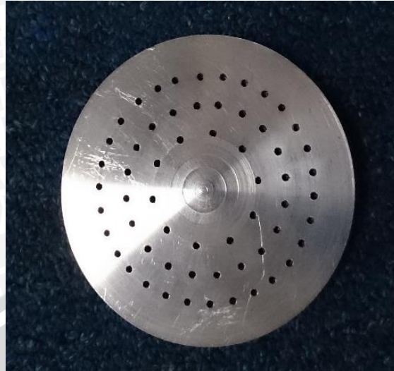
Gambar 3.7 Perforate burner material aluminium Sumber: Arsip pribadi
