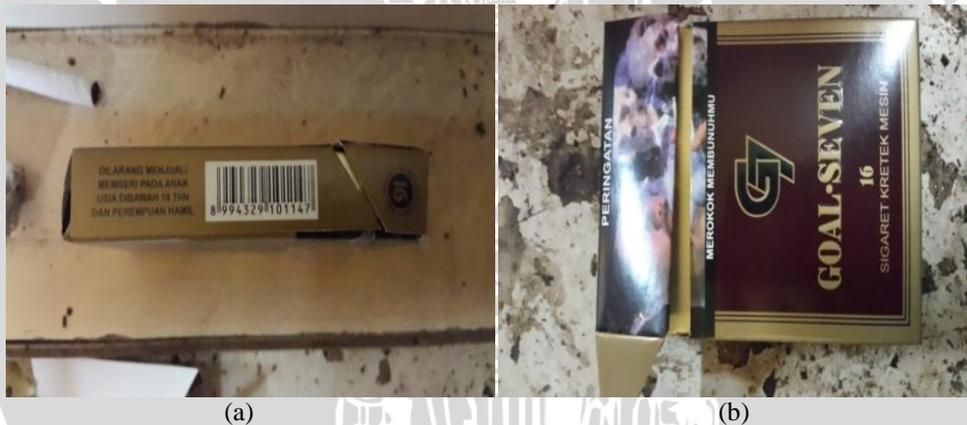
**Gambar 4.5** Cacat *packing*
