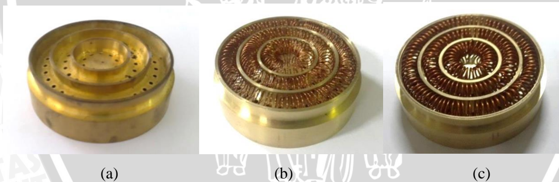
Gambar 3.1 (a) Perforated burner tanpa toroid, (b) Perforated burner dengan toroid tebal 0,5 mm, (c) Perforated burner dengan toroid tebal 1 mm
