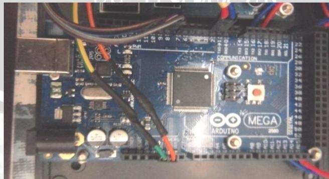
Gambar 4.6 Arduino Mega 2560
