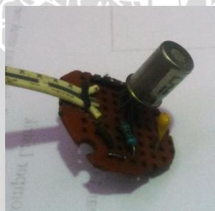
Gambar 3. 10 Sensor Gas Hidrogen
