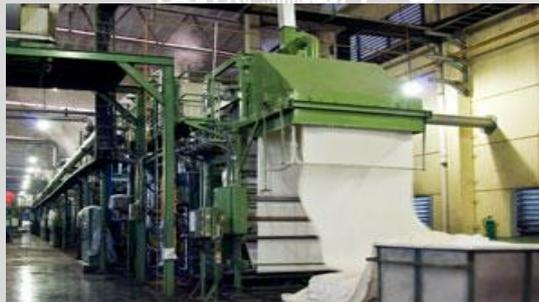
**Gambar 4.4** Mesin Continuous Bleaching
