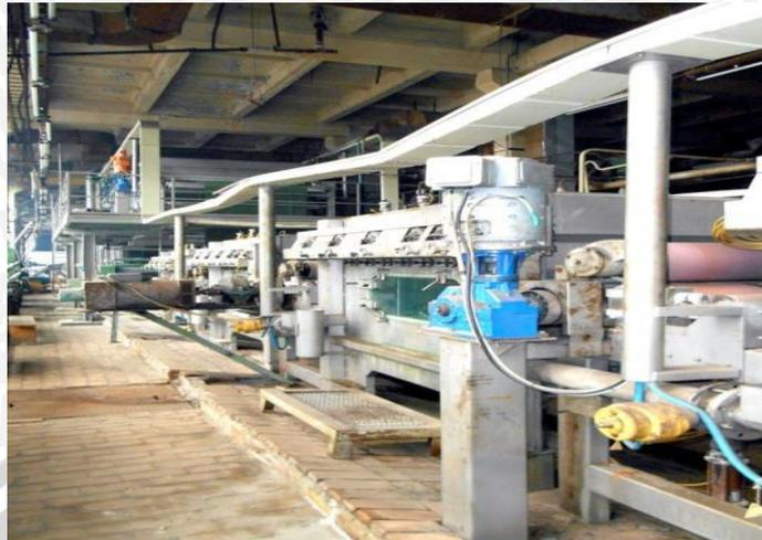
**Gambar 4.8** Mesin Pad Steamer
