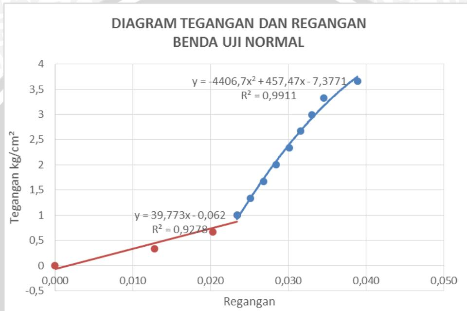
**Gambar 4.3.** Diagram tegangan-regangan benda uji normal
