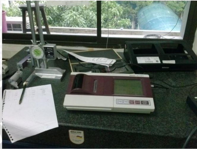
Gambar 3.2 : Surface Roughness Test
