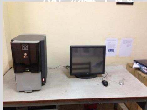
Gambar 3.14 *Scanning Electron Microscope (SEM)*
