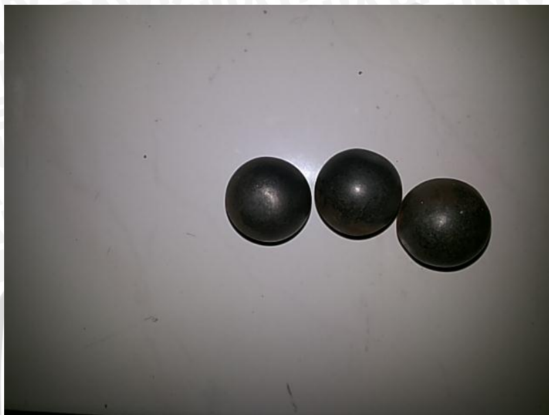
Pack carburizing temperatur 925°C holding time 45 menit
