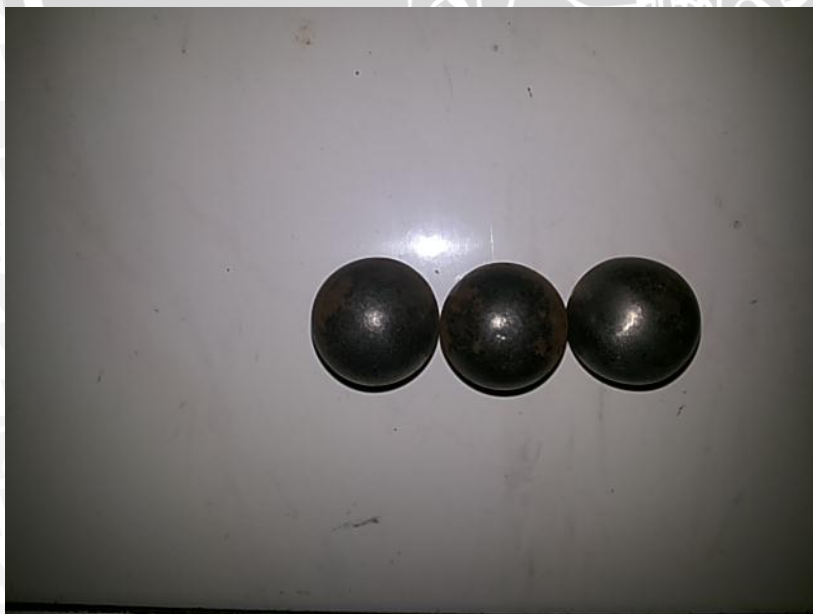
Pack carburizing temperatur 950°C holding time 60 menit
