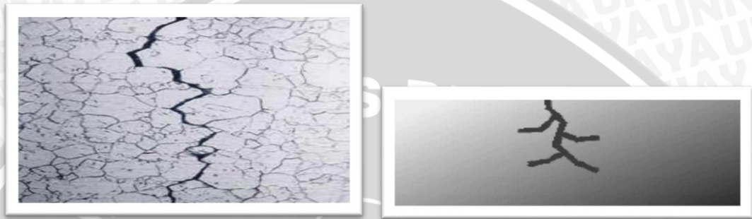
Gambar 2.19 Korosi retak tegang ( stress cracking corrosion )
