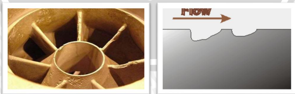
Gambar 2.18 Korosi erosi ( erosion corrosion )
