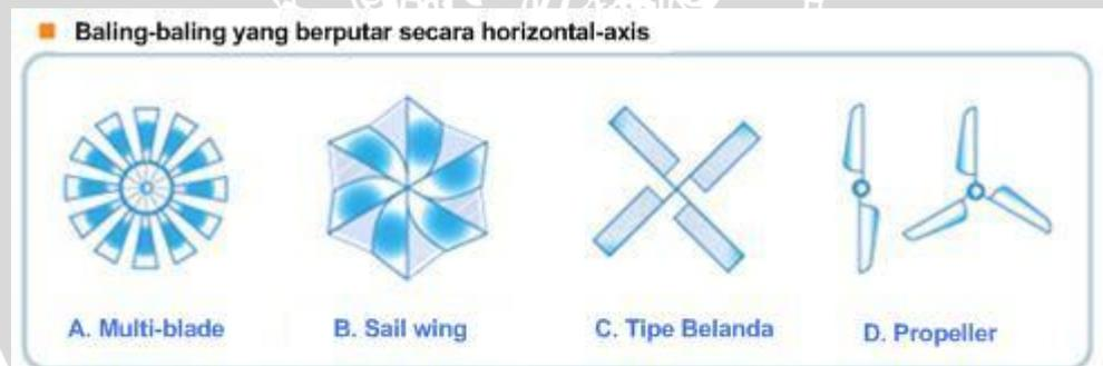
Gambar 2.4 : Turbin Angin *Horizontal Axis Wind Turbine (HAWT)*
