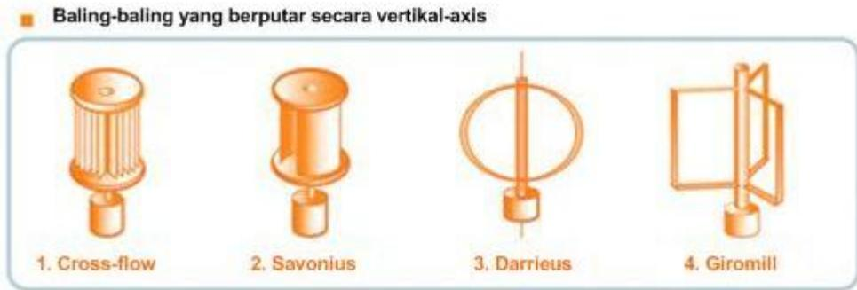
Gambar 2.5 : Turbin Angin *Vertical Axis Wind Turbine (VAWT)*
