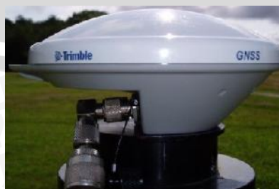
Gambar 3.4 GPS Trimble's tipe 4000ST model TRM14532.00 dual frekuensi jenis choke ring (Sumber: www.ngs.noaa.gov )
