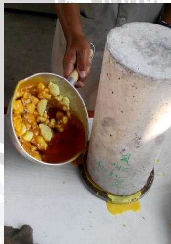
Gambar Proses Caping Silinder
