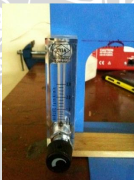
Gambar 3.9 Flow meter LPG A
