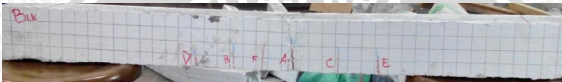
Gambar Balok Runtuh Lentur Perendaman 7 hari Kadar BA 20%
