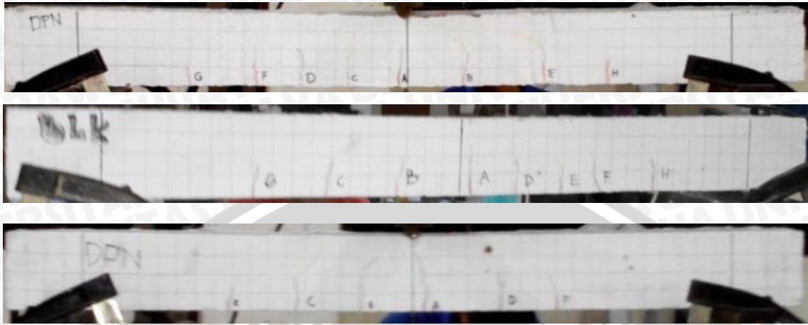
Gambar Balok Runtuh Lentur Perendaman 28 hari Kadar BA 20%
