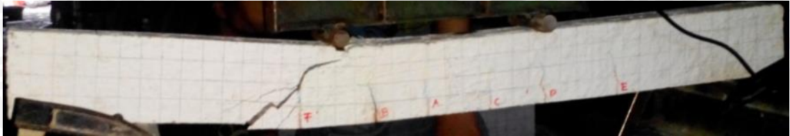
Gambar Balok Runtuh Geser Perendaman 7 hari Kadar BA 0%
