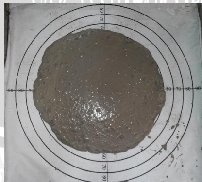
Gambar 4.3 Pengujian slump flow
