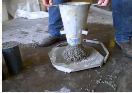
Gambar 2.7 Slump flow test
