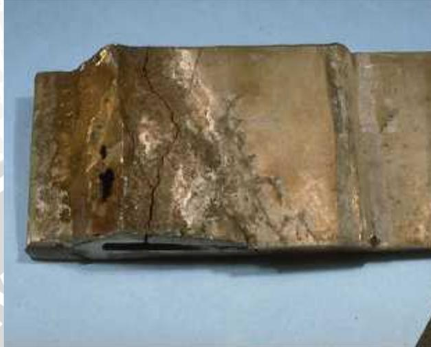
Gambar 2.10 *Stress Corrosion Cracking*
