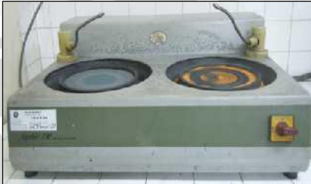
Gambar 3.4 Centrifugal sand paper machine
