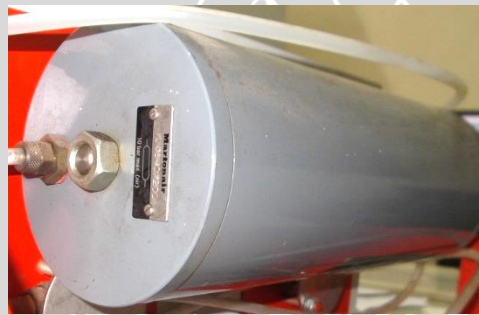
Gambar 4.3 Buffer Accumulator (Sumber: Perancangan, 2014)
