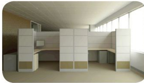
High panels impede daylight penetration.
