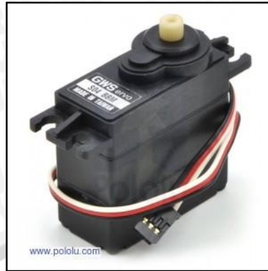
Gambar 2.3 Motor Servo (pololu.com)
