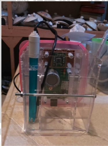
Gambar 6 sensor pH, kelembaban, CO 2 , suhu
