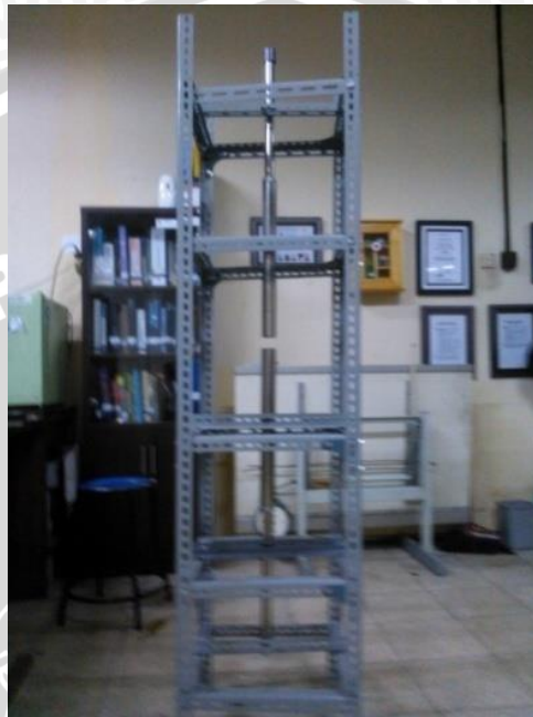
Gambar 3.1 Ruang bakar model Counterflow Flame .
