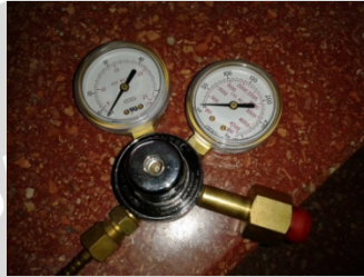
Gambar 3.6 Regulator Gas CO 2
