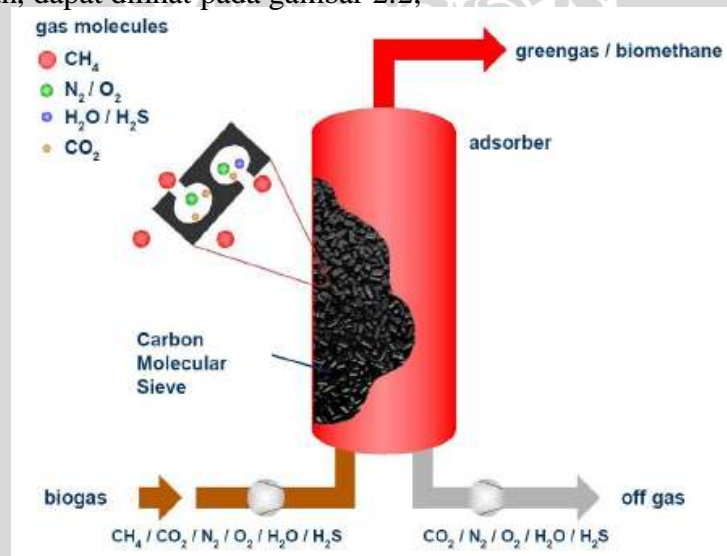
Gambar 2.2 Prinsip Kerja PSA Sumber : Hullu dkk. 2008. Comparing Diferent Biogas Upgrading Technique . Edf.
