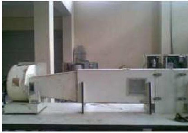
Gambar 3.3 : Wind Tunnel
