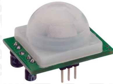
Gambar 2.4 Sensor Passive Infrared Receiver (PIR) Sumber : Yurianto, 2011:41
