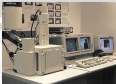
Gambar 2.14 *Scanning Electron Microscope*
