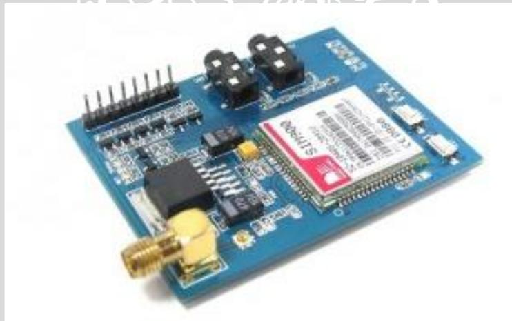
Gambar 2.5. ITEAD SIM900 GPRS/GSM *Minimum System*
