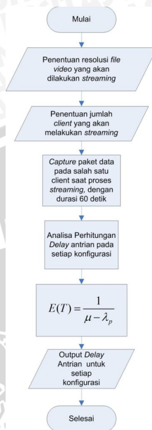
Gambar 3.11 Diagram alir perhitungan delay antrian sistem
