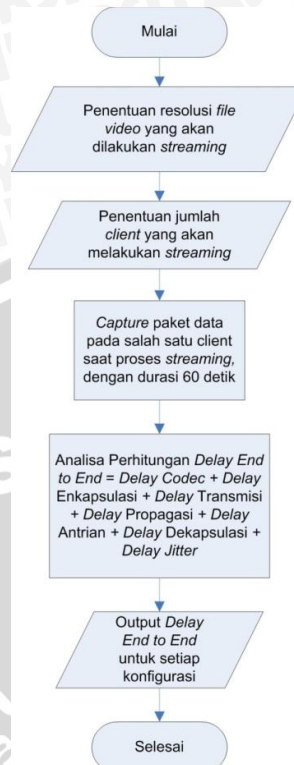
Gambar 3.5 Diagram alir perhitungan delay end-to-end sistem
