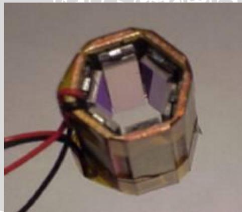
Gambar 2.9 Prototip *micro-power generator*
