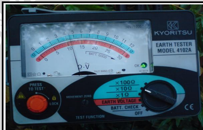
Gambar L-4. Earth Tester Resistance
