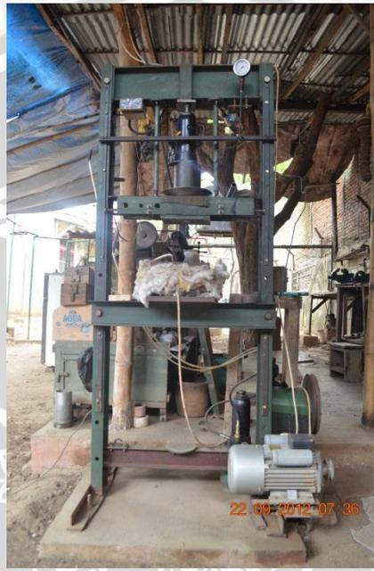
Gambar 3.1. Mesin *Hot Pressing*
