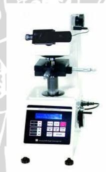
Gambar 3.14 *Micro Hardness Tester*
