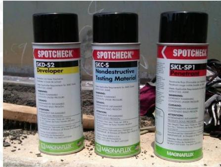
Gambar 3.11 Dye Test Penetrant
