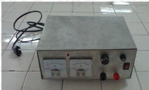
Gambar 3.3 Power Supply/ Rectifier
