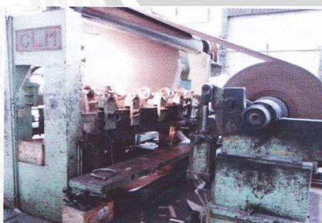
Gambar 4.29 Mesin *rewinder*
