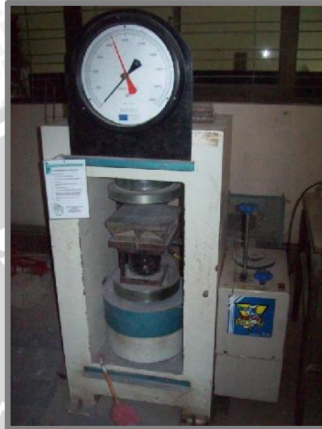
Gambar 3.1. Alat Uji Kuat Tekan (Compression Strength Testing Machine)
