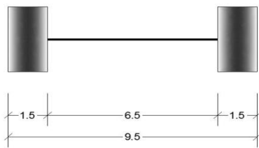
Gambar 3.6 Detail beban roda
