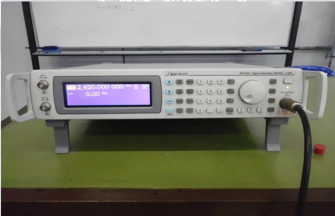
Gambar 7 Aeroflex IFR 3413 Signal Generator 250 KHz - 3 GHz
