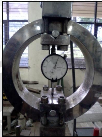
Gambar 4.16. Alat pengukur kuat lentur balok ( Proving Ring & Dial Gauge )
