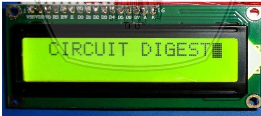
**Gambar 2. 15 LCD 16x2**
