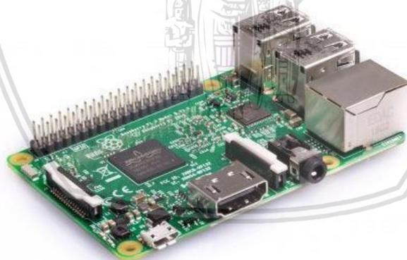
**Gambar 2. 9 Raspberry Pi 3 model B**
