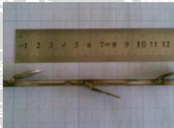
Gambar 4 Jarak antar sirip-sirip 55 mm
