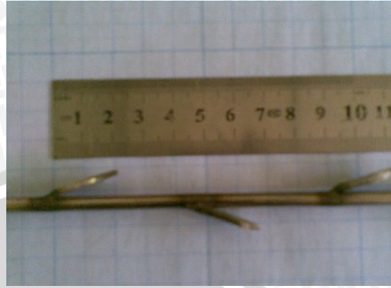
Gambar 3 Jarak antar sirip-sirip 45 mm
