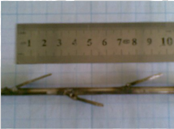
Gambar 2 Jarak antar sirip-sirip 35 mm
