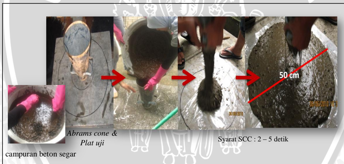
Gambar G.6 Pengujian slump flow
