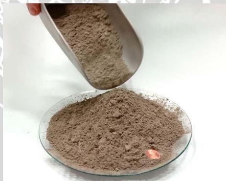
**Gambar 2.2** Fly ash tipe F
