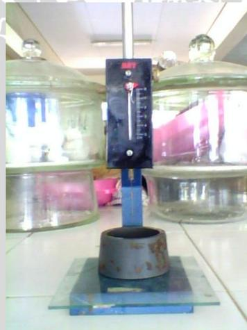
**Gambar 2.4** Vicat, alat uji *setting time*
