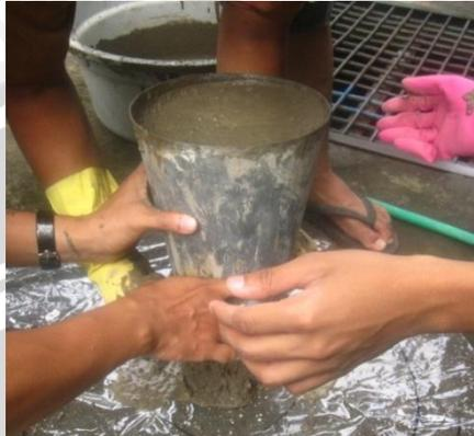
**Gambar 2.5** Pengujian *slump flow*
