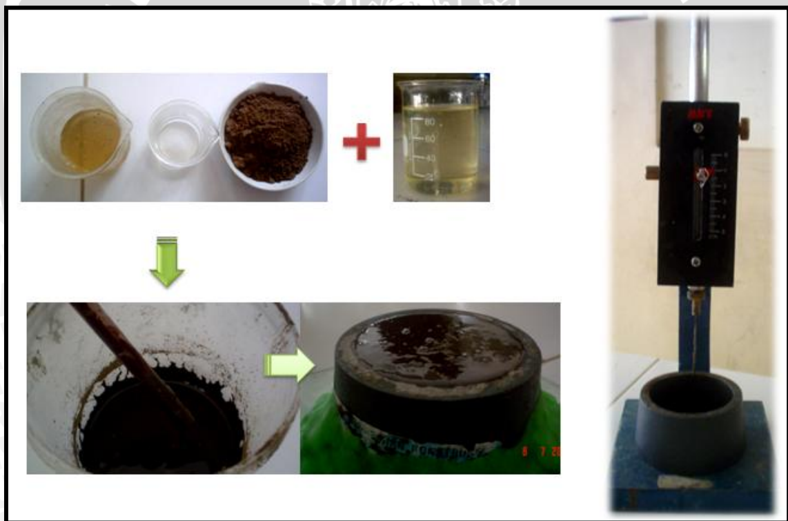
Gambar G.4 Proses pengujian setting time .
